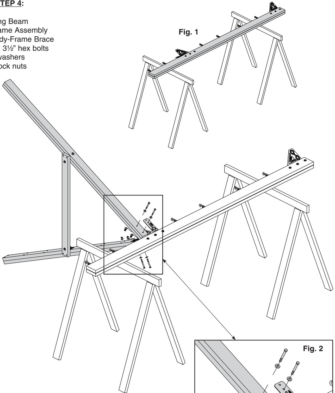
Lay swing beam on saw horses as shown. **(Fig. 1)**
