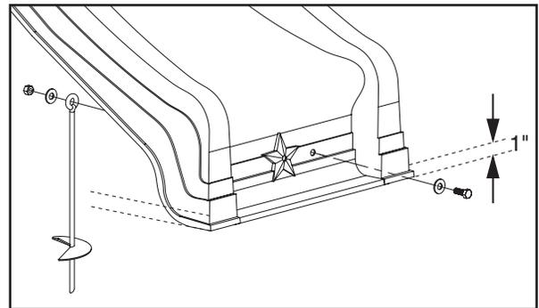
**Caution:** Failure to anchor the Slide properly could cause serious injury from children lifting the slide.
