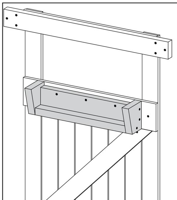
**Note:** You will want to locate Flower Box where there are thicker boards and the 2½" deck screw does not protrude through the backside.
