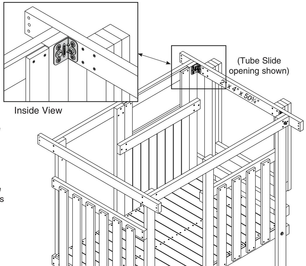
Use the bracket as a drill guide and drill <sup>1</sup>/<sub>8</sub>" holes 1" deep into the 2" x 4" x 50<sup>3</sup>/<sub>4</sub>" board. Attach with #8 x 1<sup>1</sup>/<sub>4</sub>" deck screws.
